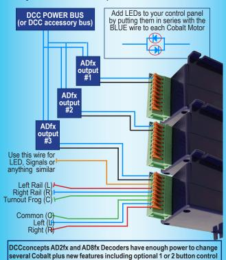
AND direct computer IO or feedback. They work well with DCC & DC too
