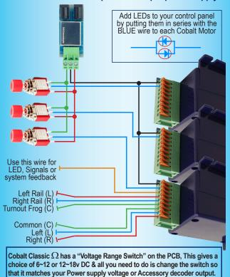
Basic wiring diagram for analog control using a more conventional single output regulated DC power supply
