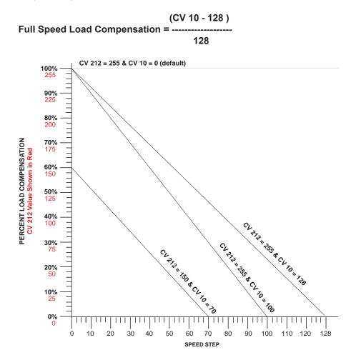
In general, you will want full load compensation at low speeds which gradually reduces to zero load compensation at full throttle and may be achieved by setting CV 10 to 126.
