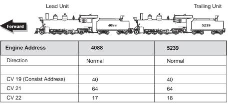
You might want the braking effect (F11) and dimmer (F7) to work on both engines. However, you will likely want the headlight (F0(f)) to only work on the lead engine, #4088, and the backup light (F0 (r)) to work only on #5239.
