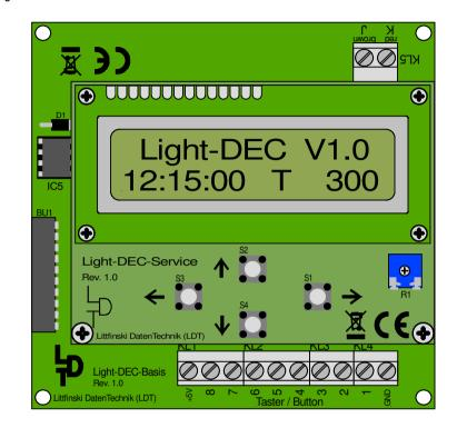
The universal layout-light-control Light-DEC consist of the Basic-Module and at-least one Light-Module (Light-Display or Light-Power) which will be plugged onto the side of the Basic-Module.
