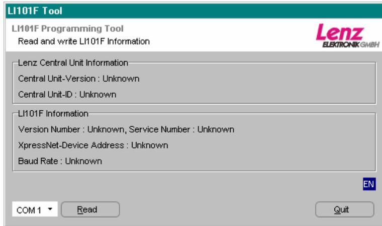
Picture 6: Display in case of faulty communication
